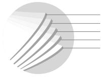
Cap Sheet- Polyester Clearcoat - Polyurethane Film - Polyurethane Adhesive - Acrylic PSA Liner - Polyester
