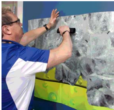
FIGURE 14 Squeegeeing Exposed Adhesive for Self Hinge
