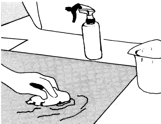
Figure 3. Flooding the Exposed Film Adhesive
